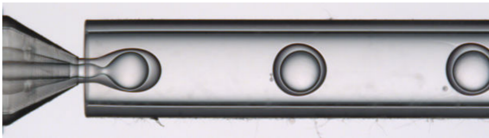
Figure 8: Generation of droplets in the Raydrop®.
