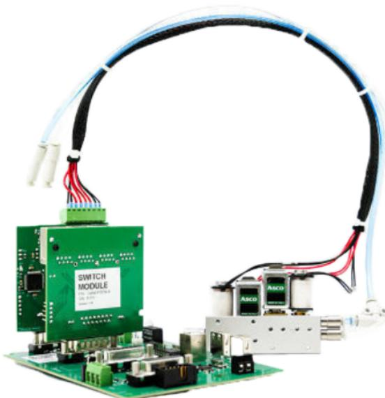
The F-OEM consists of a main platform – the integration board – that supports up to 8 modules: pressure modules (different ranges, push-pull), switch and electrovalve modules (for valve integration).
