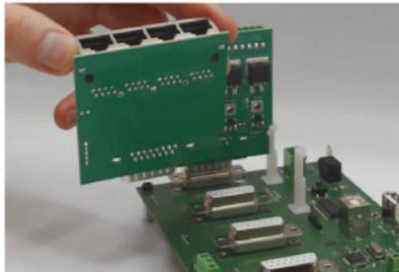
**Note:** always plug or unplug submodules while the main board is powered off.
