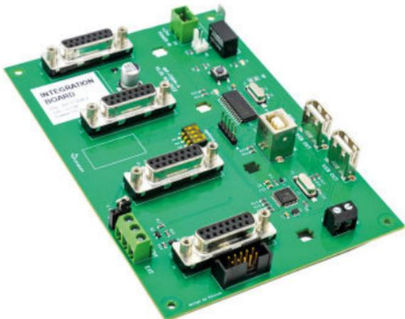
The integration board is the main platform that supports the F-OEM modules. The schematic below shows the main components of the board.
