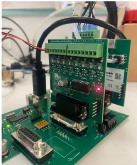
**Note:** always plug or unplug sub-modules while the main board is powered off.
