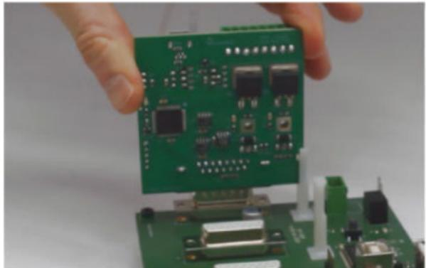
**NOTE:** make sure that the main board is powered off when plugging or unplugging submodules, as it could result in malfunctions.
