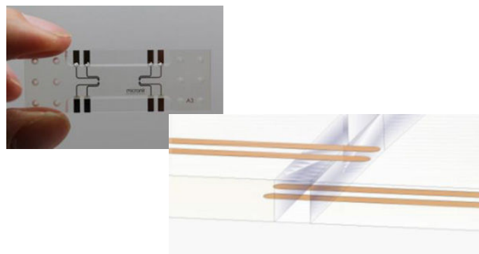
Figure 3: Electrical Impedance Spectroscopy chip from Micronit (left) Cross sectional view of electrode layout (right)
